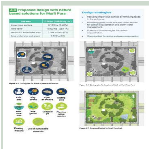
Figure 10 - Proposed design with nature-based solutions for MurliPura
