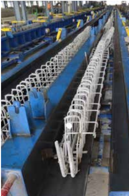
Precast Beam Casting (1800 Rmt /Day)
